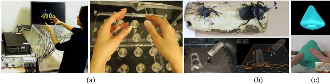
Figure 1: IM3D. (a) 3D interaction with markers fixed on user's fingers, (b) tracking motion of insects, (c) real-time 3D modeling
