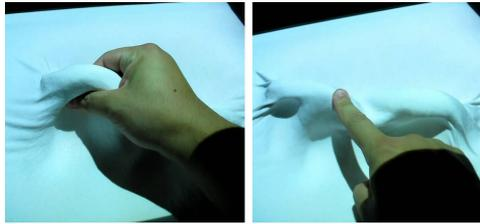
Figure 1: Surface in a Soft State(left) and Hard State(right)
