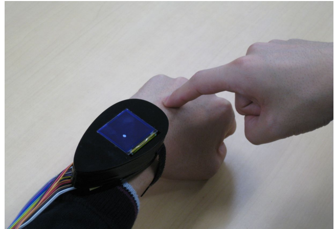
Figure 1: Touch interface device. A user can input data by touching the back of the hand. The user can feel the position of the manipulation from his/her own hand, the system do not need any tactile display device to give “touch” sensation.
