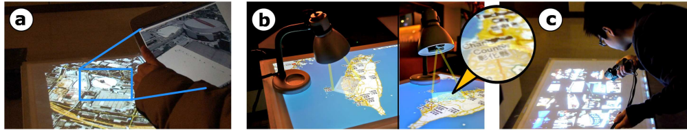
Figure 1: (a) iView enables users to explore 3D views from different perspectives above the 2D table surface. (b) iLamp highlights and enhances resolution of a particular region, (c) iFlashlight , a mobile version of iLamp , facilitates cooperative information exploration.
