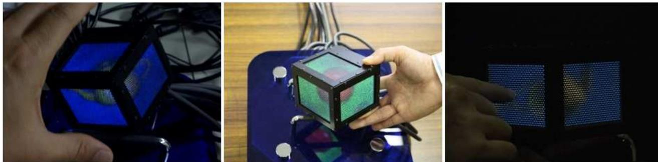
Figure 1: *gCubik* is an autostereoscopic display, graspable, interactive and suitable for multiple users
