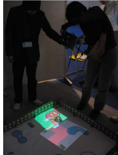
Figure 1: CoGAME: A robot navigation game using projected images given through mobile devices
