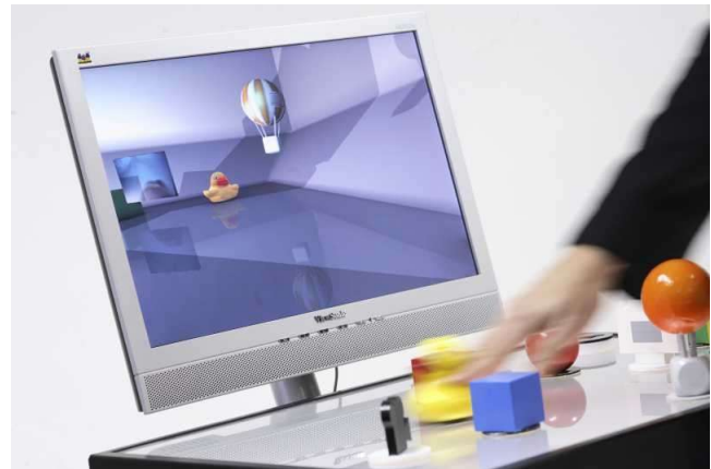
All virtual objects are controlled by moving the corresponding items on the navigation surface
