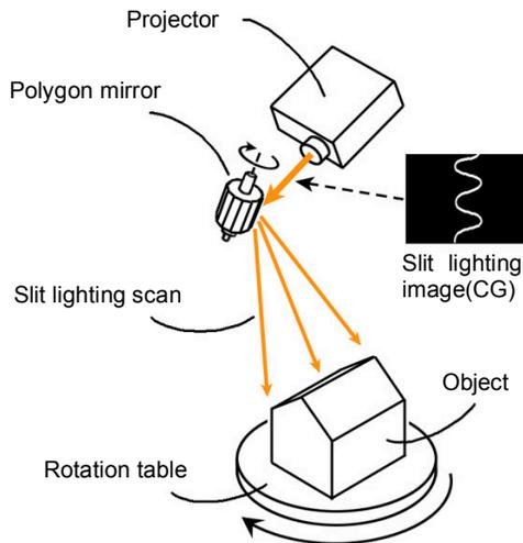
Figure 2 : System configuration
