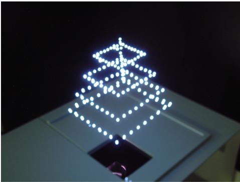
Figure 1: A 3D-object displayed using a 3D-image spatial drawing device we have developed.
