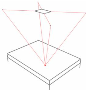
The feeler can reach any position in three-dimensional space in between the bed and the ceiling. At each moment in time, the feeler knows exactly where it is, by performing a geometrical computation based on the length of each suspension line.
