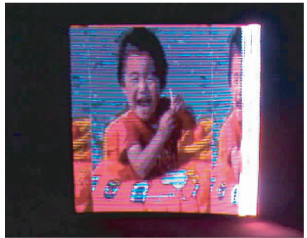
Figure 4: Full-scale color image presented with saccade-based display (this image was captured by rotating the video camera).
