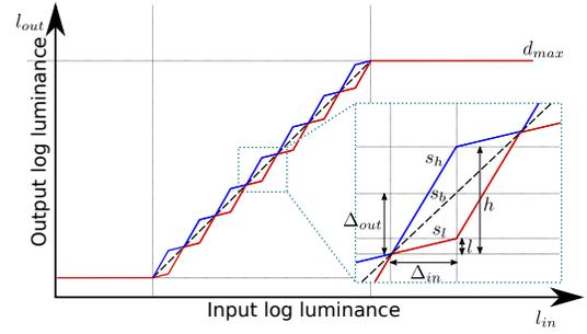
**Figure 3:** The tone-curve for the right eye shown in red and for the left eye in blue. The piece-wise curves consists of interleaved low- and high-slope segments. We denote the lower slope as  $s_l = l/\Delta_{in}$  and the higher slope as  $s_h = h/\Delta_{in}$ .
