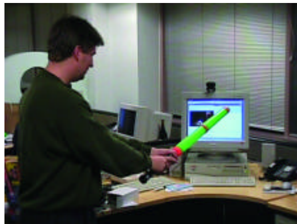
The user manipulates rendered objects by moving real objects in front of a video camera.
