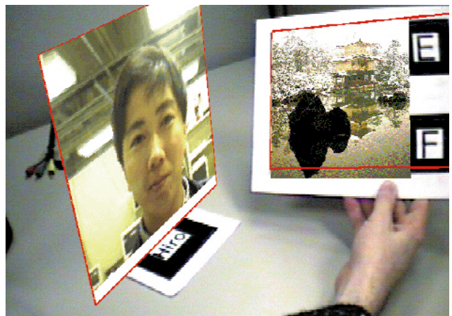
A virtual video window of a remote collaborator and shared virtual image attached to a real-world object.
