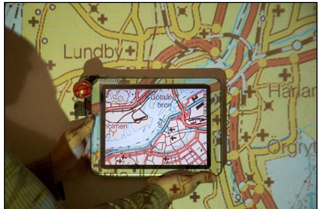
Figure 1: A user holds up a tablet PC in front of a large projected image to view details and interact with the shared workspace.
