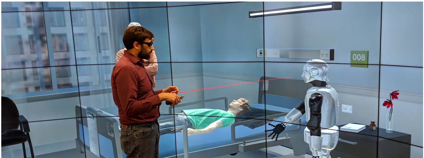
Figure 1: Using a monitor wall to talk to a virtual robot, modeled using a combination of Unity, ROS, and Gazebo.
