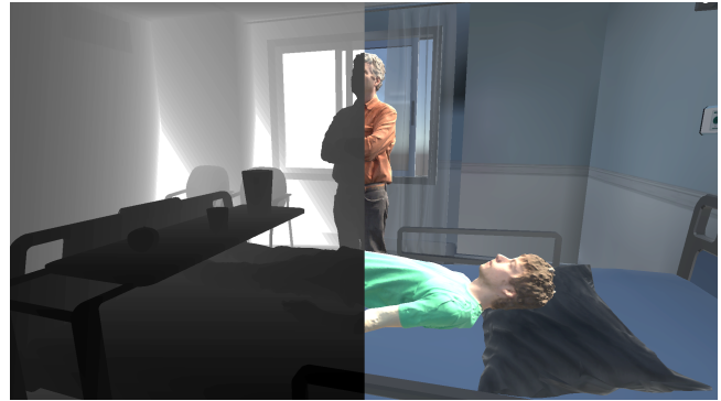
Figure 2: A split view of the robot’s perspective, with an RGB image on the right and depth sensor data on the left.
