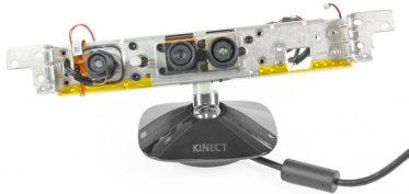
Figure 5: Multiple sensors in the Kinect camera
