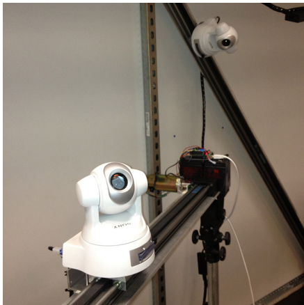
Figure 2: A close-up taken during development showing a robotic camera in the foreground and the motor driving the rail in the background.
