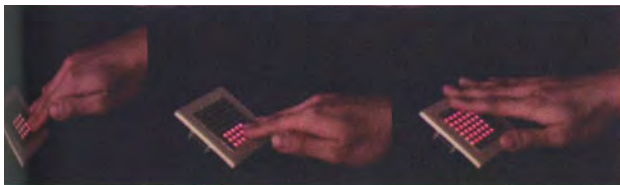
Figure 9 FishFace electric field sensing modules for non-contact, gestural input.
